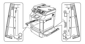
To level the machine, adjust the feet of the lower tray unit at the front and back on the right-hand side. Turn the feet to move them up or down until they touch the work surface and the tray unit is level.
