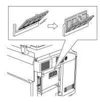
Press the SO-DIMM straight into the slot (press firmly). Make sure the locks on each side of the SO-DIMM click into place.
