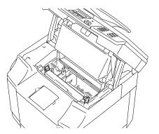
5 Remove the OPC belt cartridge from the machine, place it in the original plastic bag.
