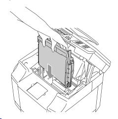
9 To lock the cartridge into the machine, push the belt cartridge lock levers that are on both sides of the OPC belt cartridge outwards.
