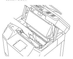
7 Put the new transfer belt cleaner into the machine by gently placing the brass bearings into the guides, and then pushing the handle down until the bearings click into place. Make sure the transfer belt cleaner is free to move slightly upwards (rotating slightly around the bearings) in the housing after you have installed it.
