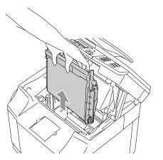
6 Open the front cover of the machine. Pull out all the toner cartridges and the waste toner pack from the machine.
