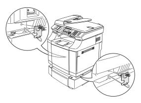
8 Cover the gap on the right hand side with the right-hand side cover by first inserting the hook at the back. Cover the gap on the left hand side with the left-hand side cover by first inserting the hook at the back.
