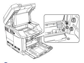
8 Remove the tape from the supplied protective sponge and cover the opening of the waste toner pack as shown in the illustration.
