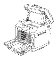
7) To avoid any toner spills, plug the waste toner hole located at the bottom right inside of the machine with the supplied protective sponge.
