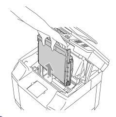
6 Place the OPC belt cartridge on a flat surface and cover the shiny green OPC belt with a piece of paper to prevent exposing it to light.
