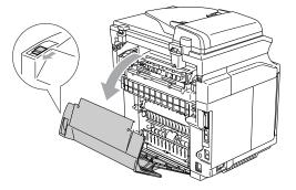
Release the transfer roller lock levers on the right and left-hand sides, and then lift the levers to release the transfer roller.
