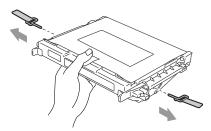
7 Remove the protective sheet from the new OPC belt cartridge. Do not touch the green part of the OPC belt cartridge.
