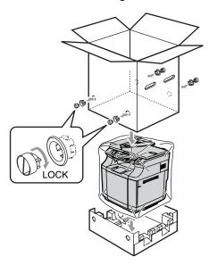
14 Put the two Styrofoam pieces on top of the machine and then put the accessory box on top of the Styrofoam.
