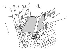
If the paper is caught in the fusing roller, release the fusing unit pressure release levers on both sides.
