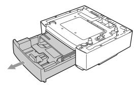
5 Remove the protective parts and then put the paper tray back in the lower tray unit.
