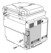
Unscrew the screw holding the metal shield plate, and then remove the metal shield plate.
