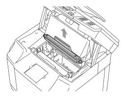
6 Clean the area where the new transfer belt cleaner is to be installed with a dry cotton cloth.
