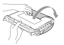
8 Put the new OPC belt cartridge into the machine guides with the flat side facing you.
