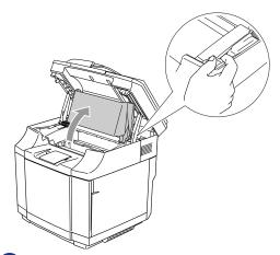
4 To release the lock, push the green belt cartridge lock levers that are on both sides inwards.
