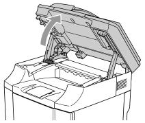
3 Open the inside cover so that it latches under the scanner unit.
