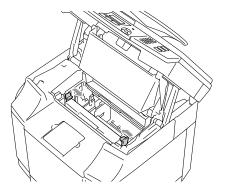
5 Remove the OPC belt cartridge from the machine.
