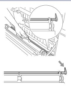
3 Clean the transfer roller unit and the transfer roller guide with a dry soft, lint-free cloth to prevent paper jams.
