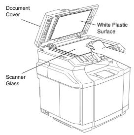
In the ADF unit, clean the white plastic bar and the scanner glass strip under it with isopropyl alcohol on a lint-free cloth.
