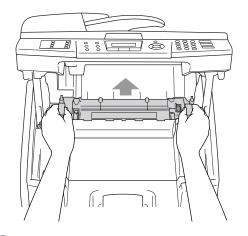
5 Put the new fusing unit into the machine. Be sure to insert the fusing unit completely into the machine.
