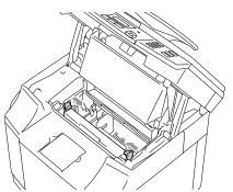
5 Remove the OPC belt cartridge from the machine.
