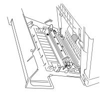
Take out the transfer roller by gently pulling the right-hand side up and sliding the transfer roller to the right.
