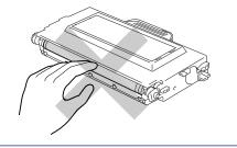
5 Put in the new toner cartridge by positioning it in the guide. Slide it gently into the machine. Do not try to push or lock the new toner cartridge in; it must rest loosely in the guide rails and will automatically be positioned properly when the front cover is closed. Note that each colour cartridge is individually keyed to prevent improper installation. Match each cartridge colour label to the same colour label on the machine.
