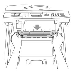
6 Secure the fusing unit with the two lock levers that are on both sides of the fusing unit.
