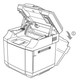
3 To release the fusing unit from the machine, release the lock levers that are on both sides of the fusing unit.
