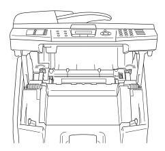
4 Hold the handles on both sides as you take the fusing unit out of the machine.
