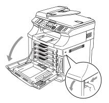
2 Remove the waste toner pack from the holder at the lower right hand side of the machine. Be careful not to spill the toner.
