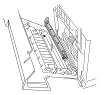
5 Put in the new transfer roller by holding the lock levers of the transfer roller and adjusting the angle of the transfer roller lever shafts (both sides) to match the transfer unit grooves. Put the transfer roller onto the shafts and place the roller onto the springs as shown below:
