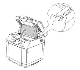
4 To release the lock, push the green belt cartridge lock levers on both sides inwards.
