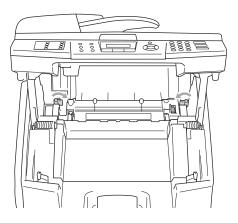
**(7)** Move the fusing unit pressure release levers to the Set position.
