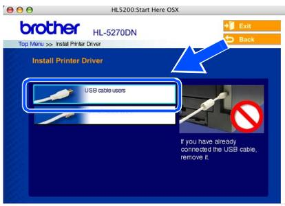
3 Connect the USB interface cable to your Macintosh®, and then connect it to the printer.
