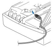
**10** Carefully guide the USB cable into the trench as shown below, following the trench around and toward the back of the machine.
