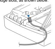
Δ Carefully guide the network cable into the trench as shown below, following the trench around and toward the back of the machine. Then, connect the cable to your network.
