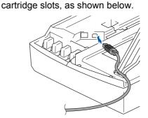
Carefully guide the USB cable into the trench as shown below, following the trench around and toward the back of the machine.
