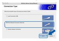
After the DeviceSelector window appears, connect the network interface cable to your Macintosh<sup>®</sup> and then to the machine.
