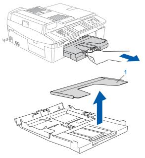
Press and slide the paper guide (1) to fit the paper width.
