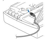
Carefully guide the USB cable into the trench as shown below, following the trench around and toward the back of the machine.
