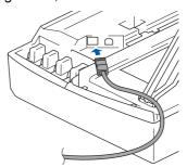
10 Carefully guide the network cable to the trench as shown below, following the trench around and toward the back of the machine.
