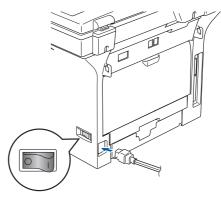
2 Plug the AC power cord into an AC outlet. Turn the power switch on.
