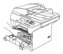
Clean the primary corona wire inside the drum unit by gently sliding the blue tab from right to left and left to right several times.
