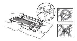
Clean the primary corona wire inside the drum unit by gently sliding the blue tab from left to right and right to left several times. Be sure to return the blue tab to the home position  $(\mathbf{\nabla})$ .
