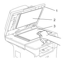
3 In the ADF unit, clean the white plastic bar (1) and the scanner glass strip (2) under it with isopropyl alcohol on a lintfree cloth.
