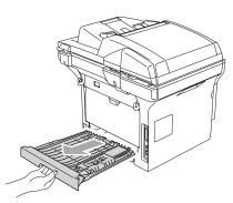
2 Pull the jammed paper out of the machine or the duplex tray.
