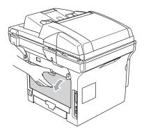
Pull the tabs at the left and right hand 4) sides toward you to open the fuser cover (1).
