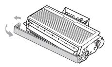
6 Put the new toner cartridge firmly into the drum unit until you hear it lock into place. If you put it in properly, the lock lever will lift automatically.
