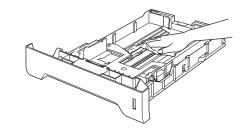
5 Re-load the paper and put the paper tray firmly back in the machine.
