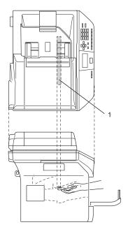
4 Put the drum unit and toner cartridge assembly back into the machine.
