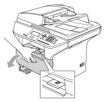
4 Slowly take out the drum unit and toner cartridge assembly. The jammed paper may be pulled out with the toner cartridge and drum unit assembly, or this may release the paper so you can pull it out of the paper tray opening.
