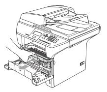
2 Clean the primary corona wire inside the drum unit by gently sliding the blue tab from right to left and left to right several times.
