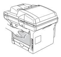
4 Pull the tabs at the left and right hand sides toward you to open the fuser cover (1).
