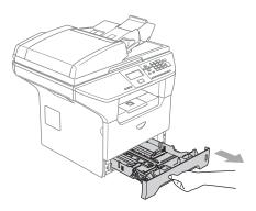
3 While pressing the blue paper-guide release lever (1), slide the paper guides to fit the paper size. Make sure that the guides are firmly in the slots.
