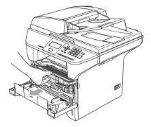
3 Hold down the lock lever on the right and take the toner cartridge out of the drum unit.
