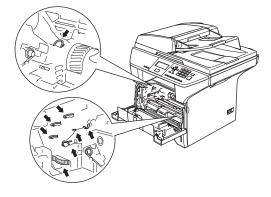
2 Hold down the lock lever on the right and take the toner cartridge out of the drum unit.
