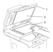
In the ADF unit, clean the white plastic bar (1) and the scanner glass strip (2) under it with isopropyl alcohol on a lintfree cloth.
