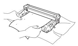
3 Turn the white gear on the drum as you check the surface of the OPC drum (1).
