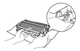
4 Put the toner cartridge back into the drum unit until you hear it lock into place. If you put it in properly, the lock lever will lift automatically.
