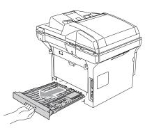
2 Pull the jammed paper out of the machine or the duplex tray.
