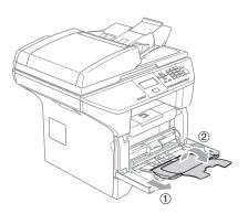
Insert the media into the MP tray with the top edge first and the printing side face up.
