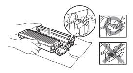
5 Put the drum unit and toner cartridge assembly back in the machine. Do not close the front cover.
