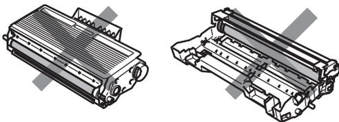
DO NOT touch the shaded parts shown in the illustrations to prevent any degradation to the print quality.
