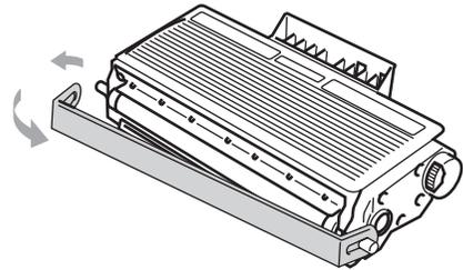
6. **6** Put the new toner cartridge firmly into the drum unit until you hear it lock into place. If you put it in properly, the lock lever will lift automatically.
