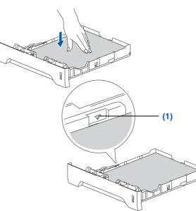
5 Put the paper tray firmly back into the machine and unfold the support flap (1) before you use the machine.
