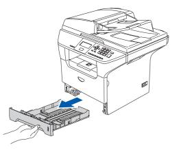
2 While pressing the blue paper guide release lever (1), slide the adjusters to fit the paper size. Check that the guides are firmly in the slots.
