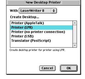
At this point we must select the correct PPD file for the machine and also configure the correct LPR information. Click Change in the PostScript Printer Description (PPD) File section and select the appropriate PPD file for your model.
