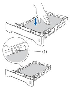
Put the paper tray firmly back into the machine and unfold the output tray support flap (1) before you use the machine.
