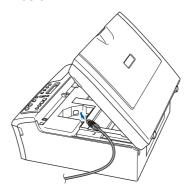
12 Carefully guide the USB cable into the trench as shown below, following the trench around and toward the back of the machine.
