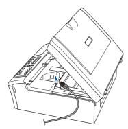
Carefully guide the USB cable into the trench as shown below, following the trench around and toward the back of the machine.
