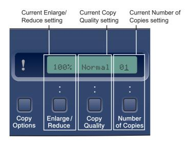
When the machine is idle (not being used) it will return to the default display shown above. The default display can give you useful information about the current settings.
