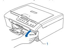
Pull all the lock release levers down and remove the yellow protective part (1).
