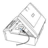
10 Carefully guide the USB cable into the trench as shown below, following the trench around and toward the back of the machine. Then connect the cable to your computer.
