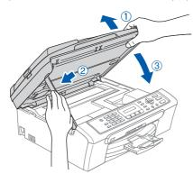
12 Turn on the machine by connecting the power
