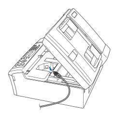
12 Carefully guide the USB cable into the trench as shown below, following the trench around and toward the back of the machine and connect it to your computer.
