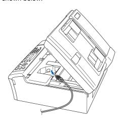
Carefully guide the USB cable into the trench as shown below, following the trench around and toward the back of the machine and connect it to your computer.
