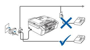
Set the receive mode to 'External TAD' if you have an external answering machine. For details, see Connecting an external TAD (telephone answering device) in Chapter 7 of the User's Guide.
