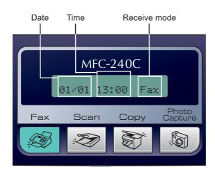
When the machine is idle (not being used) it will return to the default display shown above. The default display shows the date, time, and the current receive mode.
