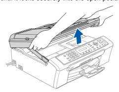
11 Insert the USB cable into the USB socket marked with a symbol. You will find the USB socket inside the machine on the right as shown below.
