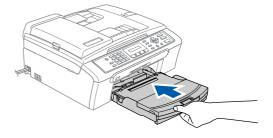
While holding the paper tray in place, pull out the paper support (1) until it clicks, and then unfold the paper support flap (2).
