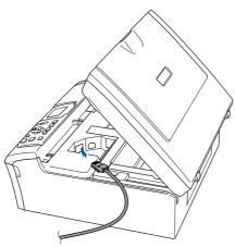
4 Carefully guide the network cable into the trench as shown below, following the trench around and toward the back of the machine. Then, connect the cable to your network.
