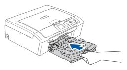
8 While holding the paper tray in place, pull out the paper support (①) until it clicks, and then unfold the paper support flap (②).
