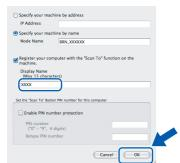
• If you want to use the machine's Scan key to scan over the network you must check the **Register** your computer with the "Scan To" function on the machine box. • The name you enter will appear on the machine's LCD when you press the **Scan** key and choose a scan option. (For more information, see Network Scanning in the Software User's Guide on the CD-ROM.)
