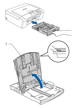
Press and slide the paper side guides (1) and paper length guide (2) to fit the paper size.
