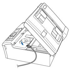
3 Carefully guide the network cable to the trench as shown below, following the trench around and toward the back of the machine. Then, connect the cable to your network.
