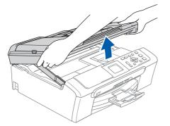
Connect the network cable to the LAN socket marked with a symbol. You will find the LAN socket inside the machine on the left as shown below.
