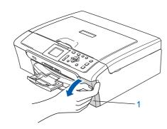
**3** Pull all the lock release levers down and remove the yellow protective part (1).
