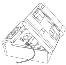
4 Carefully guide the network cable into the trench as shown below, following the trench around and toward the back of the machine. Then, connect the cable to your network.
