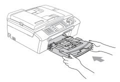
8 While holding the paper tray in place, pull out the paper support (1) until it clicks and unfold the paper support flap (2).
