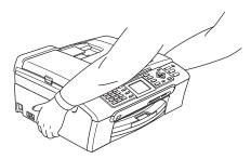
If the machine becomes hot, releases smoke, or generates any strong smells, immediately unplug the machine from the electrical socket. Call Brother dealer for service.
