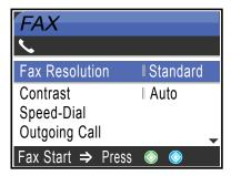
Press  $\triangle$  or  $\nabla$  to scroll through the **Fax** key options. Some functions are only available when sending monochrome faxes.
