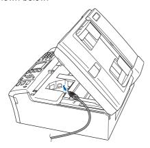
Carefully guide the USB cable into the trench as shown below, following the trench aound and toward the back of the machine. Then, connect the cable to your computer.
