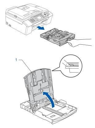
Press and slide the paper side guides (1) and paper length guide (2) to fit the paper size.
