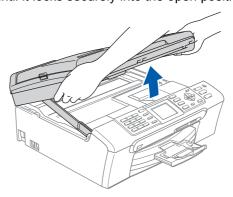
11 Connect the USB cable to the USB socket marked with a symbol. You will find the USB socket inside the machine on the right as shown below.
