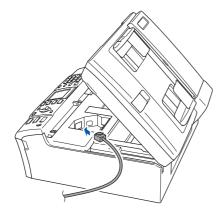
Carefully guide the network cable into the trench as shown below, following the trench around and toward the back of the machine. Then, connect the cable to your network.
