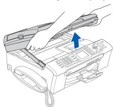
Connect the network cable to the LAN socket marked with a symbol. You will find the LAN socket inside the machine on the left as shown below.
