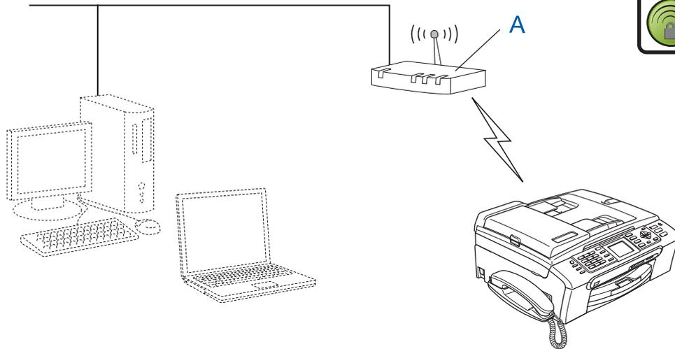
If your wireless access point (A) supports SecureEasySetup™, you do not need to use a computer to configure the machine. The access point (router) and your machine can automatically negotiate using the SecureEasySetup™ procedure.
