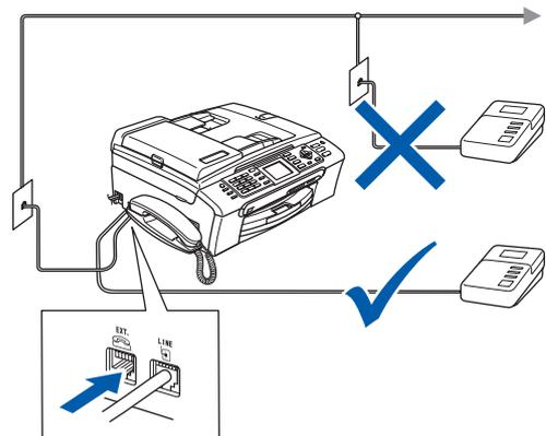
**🔍** Set the receive mode to 'Manual' if you have an external answering machine. For details, see Connecting an external TAD (telephone answering device) in Chapter 7 of the User's Guide.
