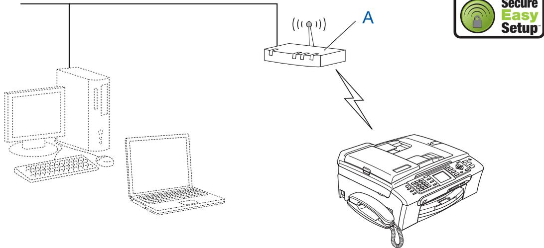
If your wireless access point (A) supports SecureEasySetup™, you do not need to use a computer to configure the machine. The access point (router) and your machine can automatically negotiate using the SecureEasySetup™ procedure.
