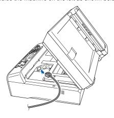
Carefully guide the network cable into the trench as shown below, following the trench around and toward the back of the machine. Then, connect the cable to your network.
