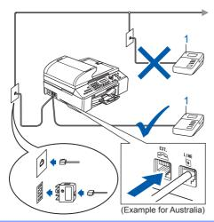
Set the receive mode to 'External TAD' if you have an external answering machine. For details, see Connecting an external TAD (telephone answering device) in Chapter 7 of the User's Guide.
