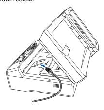
Carefully guide the USB cable into the trench as shown below, following the trench around and toward the back of the machine. Then, connect the cable to your computer.
