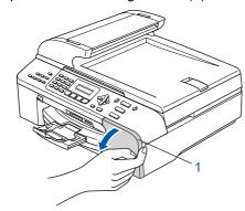
Pull all the lock release levers down and remove the yellow protective part (1).
