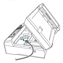
Carefully guide the network cable to the trench as shown below, following the trench around and toward the back of the machine.
