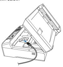
12 Carefully guide the USB cable into the trench as shown below, following the trench around and toward the back of the machine. Then, connect the cable to your computer.
