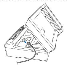
Carefully guide the network cable into the trench as shown below, following the trench around and toward the back of the machine. Then, connect the cable to your network.
