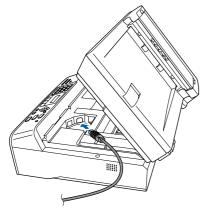
Carefully guide the USB cable into the trench as shown below, following the trench around and toward the back of the machine. Then, connect the cable to your computer.
