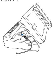
10 Carefully guide the USB cable into the trench as shown below, following the trench around and toward the back of the machine. Then, connect the cable to your computer.
