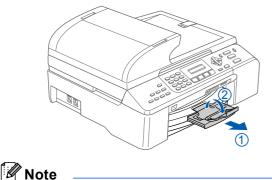
Press and slide the paper side guides (1) and paper length guide (2) to fit the paper size. Make sure that the triangular marks on the paper side guides (1) and paper length guide (2) line up with the mark for the paper size you are using.
