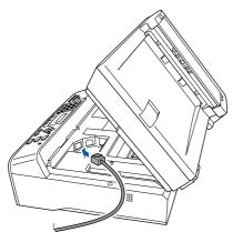
Δ Carefully guide the network cable into the trench as shown below, following the trench around and toward the back of the machine. Then, connect the cable to your network.
