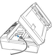
Carefully guide the network cable to the trench as shown below, following the trench around and toward the back of the machine. Then, connect the cable to your network.
