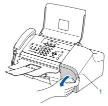
Pull all the lock release levers down and remove the yellow protective part (1).
