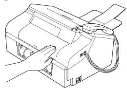
Push the paper tray firmly back into the machine. While holding the paper tray in place, pull out the paper support until it clicks and unfold the paper support. (See the illustrations in *Loading paper and other media* on page 11.)
