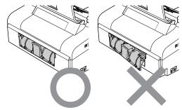
Open the Upper Jam Clear Cover (1). Make sure that there is no jammed paper left in the corners of the machine.
