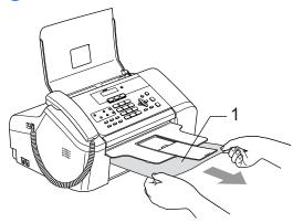
♦ If you cannot remove the jammed paper from the front side, or the error message still appears on the LCD after you remove the jammed paper, please go to the next step.
