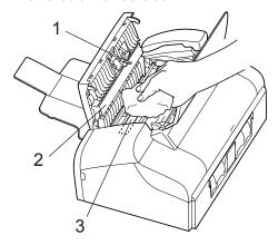
2 Soak a soft lint-free cloth with water, wring it out tightly. Wipe the whole surface of the ADF roller (1) carefully while turning it to remove dirt.
