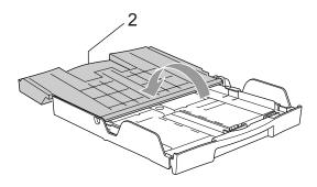
If you are using Letter, A4 or Legal size paper, press and hold the universal guide release button (1) as you slide out the front of the paper tray to match the paper size you are using.
