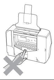
When moving the machine you must lift it from the base, by placing a hand at each side of the unit as shown in the illustration.
