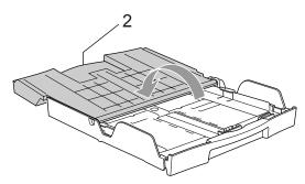
If you are using Letter, A4 or Legal size paper, press and hold the universal guide release button (1) as you slide out the front of the paper tray to match the paper size you are using.
