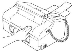
Push the paper tray firmly back into the machine. While holding the paper tray in place, pull out the paper support until it clicks and unfold the paper support.
