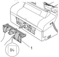
3 Clean the Paper Pick-up Roller (1) with isopropyl alcohol on a cotton swab.
