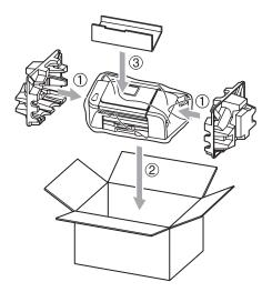
9 Pack the printed materials, and additional parts (handset, cords and CD) in the original carton as shown below. Do NOT pack the used ink cartridges in the carton.
