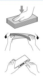
Put the envelopes or post cards into the paper tray with the address side down and the leading edge (top of the envelopes) in first. Slide the paper side guides (1) and paper length guide (2) to fit the size of the envelopes or post cards.
