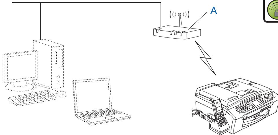
If your wireless access point (A) supports SecureEasySetup™, you do not need to use a computer to configure the machine. The access point (router) and your machine can automatically negotiate using the SecureEasySetup™ procedure.
