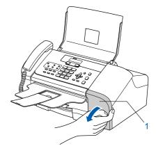
Pull the lock release lever down and remove the yellow protective part (1).
