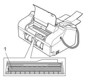
1 Clean the machine printer platen (1).
