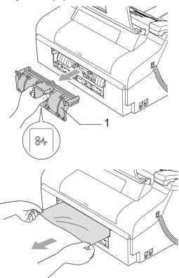
4 Put the Lower Jam Clear Cover back on. Make sure the cover is set properly.
