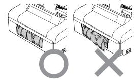
Open the Upper Jam Clear Cover (1). Make sure that there is no jammed paper left in the corners of the machine.
