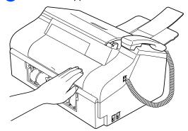
Push the paper tray firmly back into the machine. While holding the paper tray in place, pull out the paper support until it clicks and unfold the paper support (See the illustrations in *Loading* paper on page 9).
