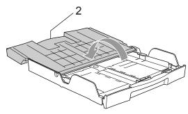
Press and hold the universal guide release button (1) as you slide out the front of the paper tray to match the paper size you are using.
