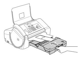
While holding the paper tray in place, pull out the paper support (1) until it clicks and unfold the paper support flap (2).
