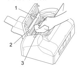
Soak a soft lint-free cloth with water, wring it out tightly. Wipe the whole surface of the ADF roller (1) carefully while turning it to remove dirt.
