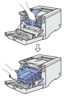
Remove the orange packing material as shown in the illustration below.
