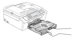
8 While holding the paper tray in place, pull out the paper support (1) until it clicks and unfold the paper support flap (2).
