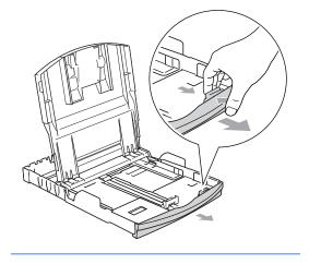
6 Gently adjust the paper side guides to the paper with both hands. Make sure the paper side guides touch the sides of the paper.
