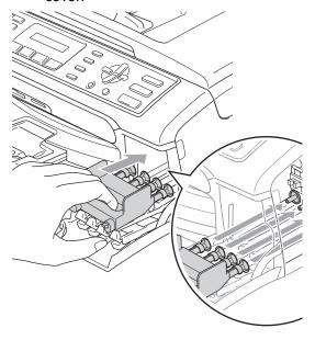
7 Lift the scanner cover (1) to release the lock. Gently push the scanner cover support down (2) and close the scanner cover (3).
