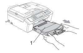
Pull out the jammed paper (1) and press **Stop/Exit**.
