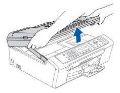
Connect the USB cable to the USB socket marked with a symbol. You will find the USB socket inside the machine as shown below.
