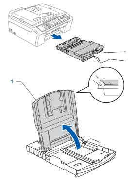
**2** Press and slide the paper side guides (1) and paper length guide (2) to fit the paper size.
