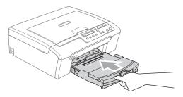
While holding the paper tray in place, pull out the paper support (1) until it clicks and unfold the paper support flap (2).
