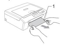
If you cannot remove the jammed paper from the front side, or the error message still appears on the LCD after you remove the jammed paper, please go to the next step. Remove the Jam Clear Cover (1). Pull the jammed paper out of the machine.
