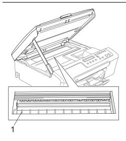
1 Clean the machine printer platen (1) and the area around it, wiping off any scattered ink with a soft, dry, lint-free cloth.
