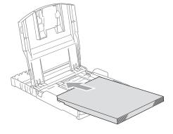
Gently adjust the paper side guides to the paper with both hands. Make sure the paper side guides touch the sides of the paper.
