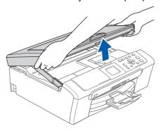
11 Connect the USB cable to the USB socket marked with a symbol. You will find the USB socket inside the machine as shown below.
