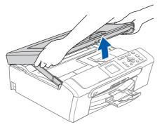
2 Connect the USB cable to the USB socket marked with a i ← symbol. You will find the USB socket inside the machine as shown below.
