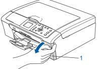
**3** Pull all the lock release levers down and remove the yellow protective part (1).
