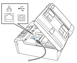
Carefully guide the network cable to the trench as shown below, following the trench around and toward the back of the machine. Then, connect the cable to your network.
