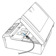
Carefully guide the USB cable into the trench as shown below, following the trench around and toward the back of the machine. Then, connect the cable to your Macintosh<sup>®</sup>.
