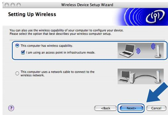
If you are using a wired computer, choose **This computer uses a network cable to connect to the wireless network.**, you must configure the wireless settings from the control panel. Click **Next** and follow the on-screen instructions to complete the setup. See *Using the Setup Wizard from the control panel* on page 22.
