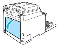
4 Pull down the two green levers, one on the left-hand-side and one on the right-hand-side, as shown in the illustration below, and then fold down the fuser cover (1).
