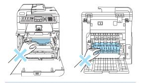
5 Using both hands, gently pull the jammed paper out of the fuser unit.
