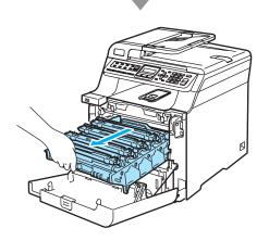
4 Release the grey lock lever (1) that is on the left side of the machine. Lift the front of the drum unit and pull the drum unit completely out of the machine using the green handles on the drum unit.
