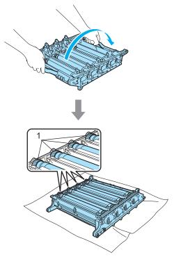
7 See the print sample to identify the colour causing the problem. The colour of the spots is the colour of the drum you should clean. For example, if the spots are cyan, you should clean the drum for cyan. Put the print sample in front of the drum, and the find the exact position of the repeating mark.
