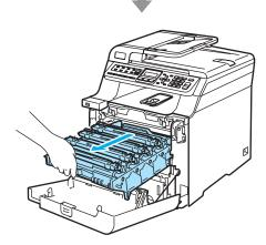
4 Using their coloured handles to lift them out, remove all four toner cartridges from the drum unit.
