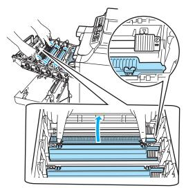
Repeat step 1 through step 3 to clean each of the remaining three corona wires. 5 Unpack the new toner cartridge. Hold the cartridge with both hands and gently shake it five or six times to spread the toner evenly inside the cartridge.
