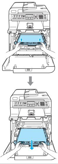
We recommend that you place the belt unit on a clean, flat surface with a piece of disposable paper underneath it in case you accidentally spill or scatter toner. 5 Remove the waste toner box from the machine using the green handle.
