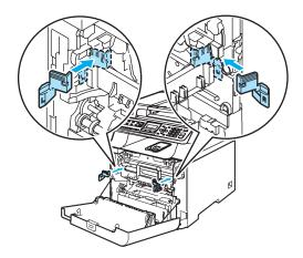
14 Two people should place the machine into the plastic bag and put the machine on the styrofoam pieces (1) in the lower carton (2). Put the upper carton (3) over the machine and the lower carton. Match the joint holes (4) of the upper carton to the joint holes (5) of the lower carton.
