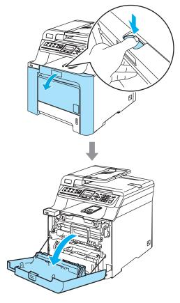
2 Hold the green handle of the drum unit. Lift the drum unit up and then pull it out until it stops.
