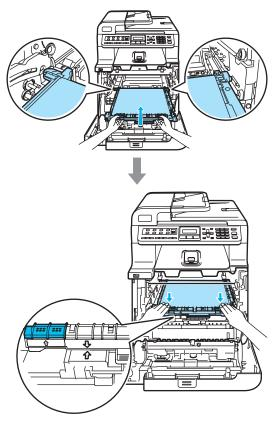
10 Insert the original orange packing material for locking the belt unit as shown in the illustration.
