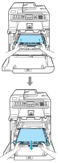
We recommend that you place the belt unit on a clean, flat surface with a piece of disposable paper underneath it in case of you accidentally spill or scatter toner. 8 Remove the waste toner box from the machine using the green handle and place it into the plastic bag included in the carton.
