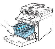
3 Hold the handle of the toner cartridge and pull it out of the drum unit. Repeat this for all the toner cartridges.
