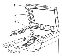
3 In the ADF unit, clean the white bar (1) and the scanner glass strip (2) underneath it with a soft lint-free cloth moistened with a non-flammable glass cleaner.
