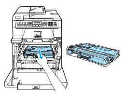
9 Put the belt unit back in the machine. Match the 1 mark on the belt unit to the t mark on the machine. Push down on the green area of the belt unit to lock it in place.
