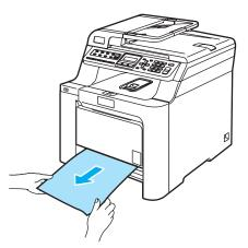
3 Make sure the paper is below the maximum paper mark. While pressing the green paper-guides release lever, slide the paper guides to fit the paper size. Make sure that the guides are firmly in the slots.
