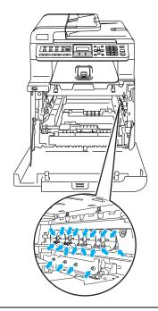
Make sure that you use the drum unit handles when carrying it. DO NOT hold the sides of the drum unit.
