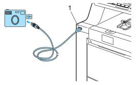
Turn on the camera. Make sure your camera is in PictBridge mode. When the machine has recognized the camera, the LCD shows the following message depending on which mode the machine is in:
