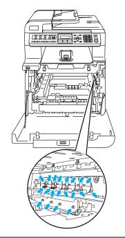
Handle the toner cartridges carefully. If toner scatters on your hands or clothes, wipe or wash it off with cold water at once. To avoid print quality problems, DO NOT touch the shaded parts shown in the illustrations.
