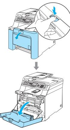
2 Hold the green handle of the drum unit. Lift the drum unit up and then pull it out until it stops.
