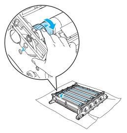
Holding the toner cartridges by their coloured handles, insert them one by one back into the drum unit as shown. Make sure that you match the toner cartridge colour to the same colour label on the drum unit, and make sure that you fold down the toner cartridge handle (A) once the toner cartridge is in place. Repeat this for all the toner cartridges.
