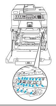
Hold the green parts of the belt unit with both hands and lift the belt unit up, then pull it out.
