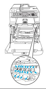
4 Hold the green parts of the belt unit with both hands and lift the belt unit up, then pull it out.
