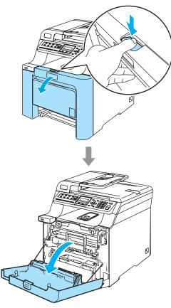
4 Hold the green handle of the drum unit. Lift the drum unit up and then pull it out until it stops.
