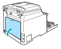
8 Put the drum unit and toner cartridge assembly back in the machine.
