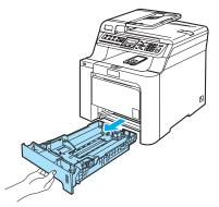
3 While pressing the green paper-guide release lever (1), slide the paper guides to fit the paper size. Make sure that the guides are firmly in the slots.
