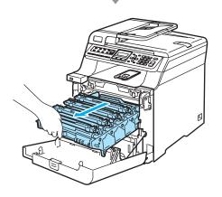
3 Release the grey lock lever (1) that is on the left side of the machine. Lift the front of the drum unit and pull the drum unit completely out of the machine using the green handles on the drum unit.
