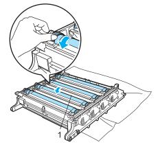
9 When you have found the mark on the drum that matches the print sample, wipe the surface of the drum gently with a cotton swab until the dust or paper powder on the surface comes off.
