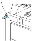
When the machine has recognized the USB flash memory drive, the **Direct** LED turns blue. Press the Direct key.
