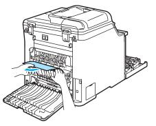
6 Close the fuser cover (1) and lift the two green levers at the left and right hand sides.
