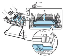
2 Clean the corona wire inside the drum unit by gently sliding the green tab from left to right and right to left several times.
