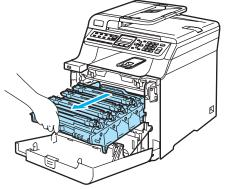
3 Release the grey lock lever (1) that is on the left side of the machine. Lift the front of the drum unit and pull the drum unit completely out of the machine using the green handles on the drum unit.
