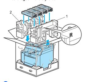
16 Put the carton tray (1) on the top. Match the front side of the machine to the  $\Delta$ marks on the carton tray. Place the waste toner box in the right side of the carton tray.
