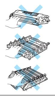
6 While holding both hands, turn the drum unit upside down and place on a piece of disposable paper or cloth. Make sure that the drum unit gears (1) are on your left hand side.
