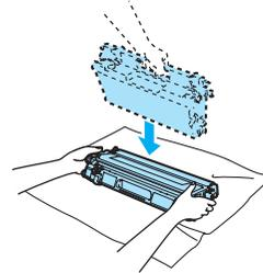
To prevent damage to the machine from static electricity, DO NOT touch the electrodes shown in the illustration.
