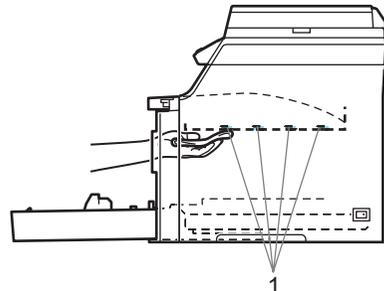
6 Put the drum unit back in the machine as follows.
