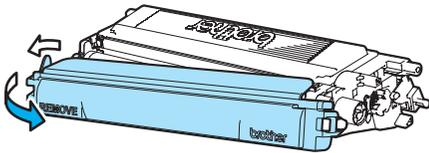
7. Hold the handle of the toner cartridge and slide the toner cartridge into the drum unit. Make sure that you match the toner cartridge color to the same color label on the drum unit, and make sure that you fold down the toner cartridge handle (A) once the toner cartridge is in place. Repeat this for all the toner cartridges.
