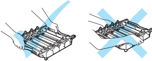
We recommend that you place the drum unit on a clean, flat surface with a piece of disposable paper underneath it in case you accidentally spill or scatter toner.
