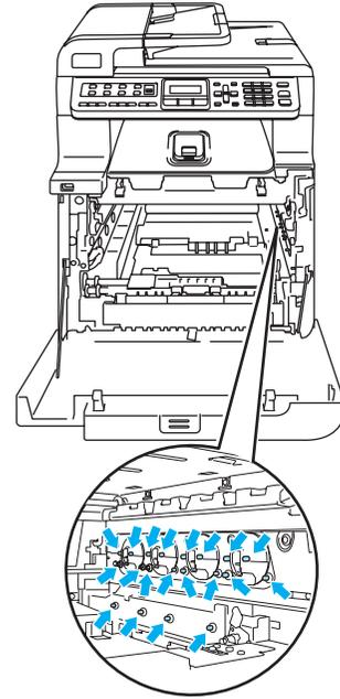
Hold the handles of drum unit when you carry it. **DO NOT** hold the sides of the drum unit.
