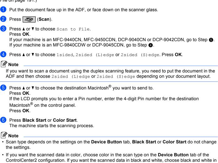
• If you would like to change the file name of scanned documents, enter the file name in **File Name** section on the Device Button tab of the ControlCenter2 configuration.
