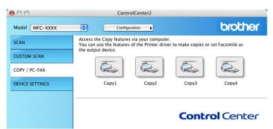
To use the Copy buttons, configure the printer driver by clicking the button while holding down the Ctrl key.
