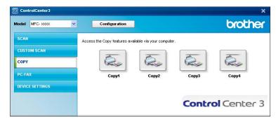
To use the **Copy** buttons, configure the printer driver by right-clicking the button and choosing the **ControlCenter Configuration**.
