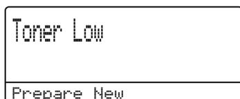
The machine is supplied with the Standard TN-150 toner cartridge. When a toner cartridge is running low, the LCD shows Toner Low.
