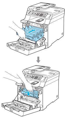
13 Insert the original orange packing material for the drum unit until as shown in the illustration, and then close the front cover.
