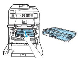
9 Put the belt unit back in the machine. Match the 1 mark on the belt unit to the 1 mark on the machine. Push down on the green area of the belt unit to lock it in place.
