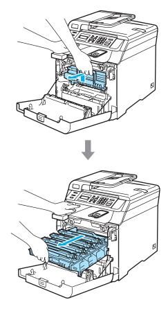
4 Release the grey lock lever (1) that is on the left side of the machine. Lift the front of the drum unit and pull the drum unit completely out of the machine using the green handles on the drum unit.
