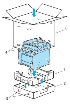
15 Put the two styrofoam pieces for the toner cartridges on the top of the machine. Match the right side of the machine to the "R" mark on one of the styrofoam pieces (1), and the left side of the machine to the "L" mark on the other styrofoam piece (2). Put the toner cartridges in the styrofoam.
