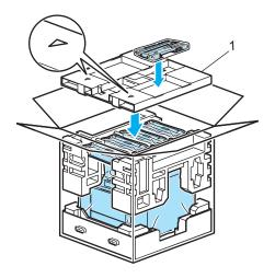
17 Put the four joints (1) into the holes of the carton using steps A and B as shown below.
