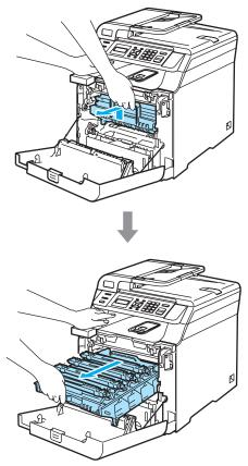
5 Release the grey lock lever (1) that is on the left side of the machine. Lift the front of the drum unit up and pull the drum unit completely out of the machine using the green handles on the drum unit.
