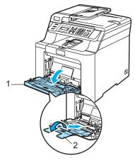
Put a blank sheet of A4 or Letter sized paper in the MP tray.
