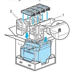
Put the two carton trays (1) on the top. Match the front side of the machine to the ∆ marks on the carton tray. Place the waste toner box in the right side of the carton tray.
