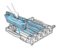
We recommend that you place the toner cartridges on a clean, flat surface with a piece of disposable paper underneath it in case you accidentally spill or scatter toner.
