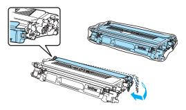
7 Hold the green parts of the belt unit with both hands and lift the belt unit up, then pull it out.
