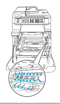
4 Hold the green parts of the belt unit with both hands and lift the belt unit up, then pull it out.
