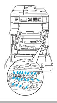
Hold the green parts of the belt unit with both hands and lift the belt unit up, then pull it out.
