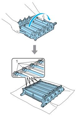
See the print sample to identify the colour causing the problem. The colour of the spots or toner stain is the colour of the drum you should clean. For example, if the spots are cyan, you should clean the drum for cyan. Put the print sample in front of the drum, and the find the exact position of the repeating mark.
