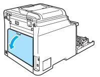
Pull down the two green levers, one on the left-hand-side and one on the righthand-side, as shown in the illustration below, and then fold down the fuser cover (1).
