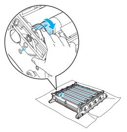
20 Holding the toner cartridges by their coloured handles, insert them one by one back into the drum unit as shown. Make sure that you match the toner cartridge colour to the same colour label on the drum unit, and make sure that you fold down the toner cartridge handle (A) once the toner cartridge is in place. Repeat this for all the toner cartridges.
