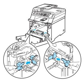
1 Put a piece of paper (letter or A4) on the belt unit to prevent damage to the belt unit.
