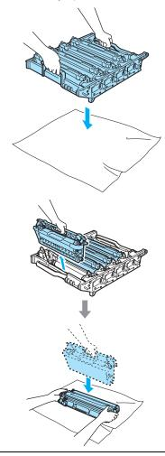
Make sure that you use the drum unit handles when carrying it. DO NOT hold the sides of the drum unit.
