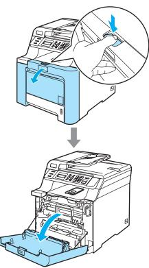
3 Hold the green handle of the drum unit. Lift the drum unit up and then pull it out until it stops.
