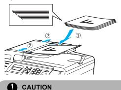
To avoid damaging your machine while using the ADF, DO NOT pull on the document while it is feeding.
