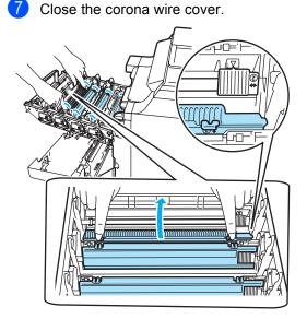
8 Repeat 6 to 7 to clean each of the remaining corona wires. There are four corona wires in total.
