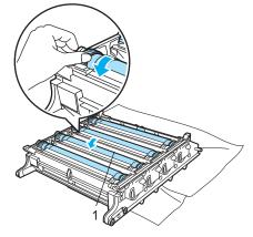
18 When you have found the mark on the drum that matches the print sample, wipe the surface of the drum gently with a cotton swab until the dust or paper powder on the surface comes off.
