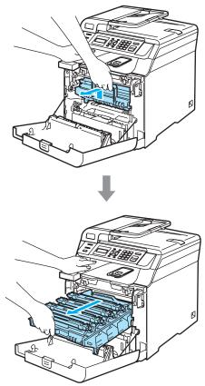
3 Hold the handle of the toner cartridge and pull it out of the drum unit. Repeat this for all the toner cartridges.
