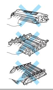
(15) While holding both hands, turn the drum unit upside down and place on a piece of disposable paper or cloth. Make sure that the drum unit gears (1) are on your left hand side.
