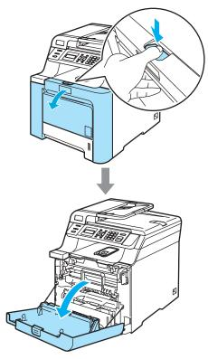
12 Hold the green handle of the drum unit. Lift the drum unit up and then pull it out until it stops.
