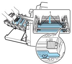
2 Clean the corona wire inside the drum unit by gently sliding the green tab from left to right and right to left several times.
