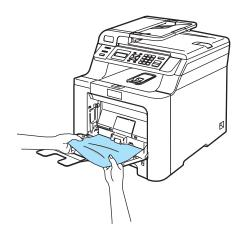
3 Close the MP tray. Then, open the front cover and close it to reset the machine. Open the MP tray again.
