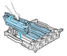
5 Unpack the new drum unit and remove the protective cover.
