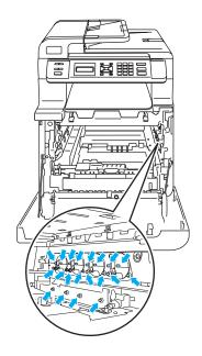
Handle the toner cartridges carefully. If toner scatters on your hands or clothes, wipe or wash it off with cold water at once. To avoid print quality problems, DO NOT touch the shaded parts shown in the illustrations.
