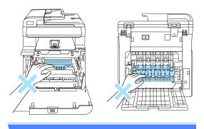
1 Turn off the machine's power switch. Press the front cover release button and then open the front cover.
