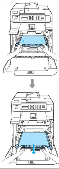
We recommend that you place the belt unit on a flat surface protected by a piece of disposable paper or cloth in case of toner scatter or spillage.
