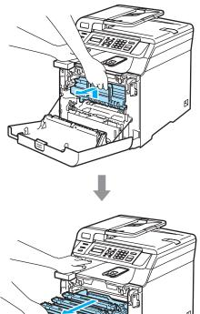
Using their coloured handles to lift them out, remove all four toner cartridges from the drum unit.
