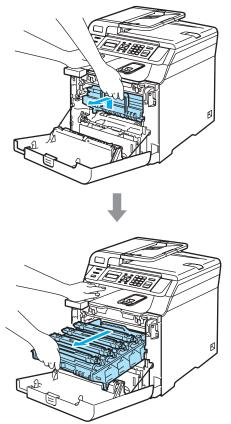
3 Release the grey lock lever (1) that is on the left side of the machine. Lift the front of the drum unit and pull the drum unit completely out of the machine using the green handles on the drum unit.
