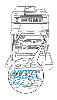
Make sure that you use the drum unit handles when carrying it. DO NOT hold the sides of the drum unit.
