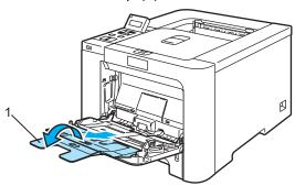
4 Lift up the support flap to prevent paper from sliding off the face-down output tray, or remove each page as soon as it comes out of the printer.
