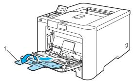
4 Lift up the support flap to prevent paper from sliding off the face-down output tray, or remove each page as soon as it comes out of the printer.
