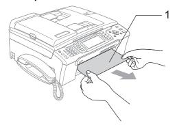
If you cannot remove the jammed paper from the front side, or the error message still appears on the LCD after you remove the jammed paper, please go to the next step. 3 Remove the Jam Clear Cover (1) from the back of the machine. Pull the jammed paper out of the machine.
