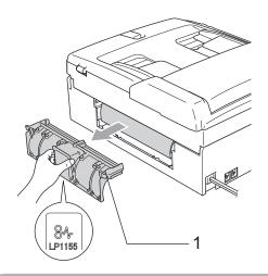
DO NOT place the jam clear cover face down as shown in the illustration. Doing this may damage the cover and cause paper jams.
