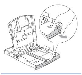
5 Gently adjust the paper side guides to the paper with both hands. Make sure the paper side guides touch the sides of the paper.
