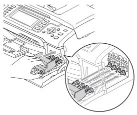
If you are not able to find the yellow protective part, DO NOT remove the ink cartridges before shipping. It is essential that the machine be shipped with either the yellow protective part or the ink cartridges in position. Shipping without them will cause damage to your machine and may void your warranty.
