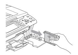
3 Open the new ink cartridge bag for the colour shown on the LCD, and then take out the ink cartridge.
