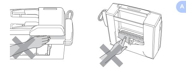
When moving the machine you must lift it from the base, by placing a hand at each side of the unit as shown in the illustration. DO NOT carry the machine by holding the scanner cover.
