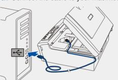
· DO NOT connect the machine to a USB port on a keyboard or a non-powered USB hub. Connect the machine directly to your Macintosh®.
