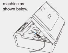
C. Carefully guide the USB cable into the cable channel and out the back of the
