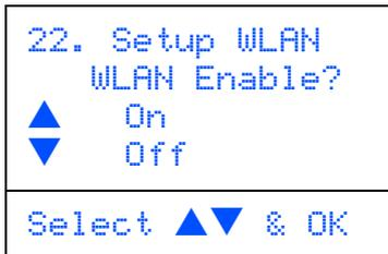
Press  or  to choose **On**, then press **OK**. The wired network interface will become inactive with this setting.
