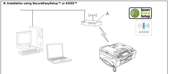
If your wireless access point (A) supports SecureEasySetup  $^{\text{TM}}$  or AOSS  $^{\text{TM}}$ , you do not need to use a computer to configure the machine. The access point (router) and your machine can automatically negotiate using the SecureEasySetup™ or AOSS™ procedure.
