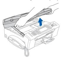
11 Connect the USB cable to the USB socket marked with a symbol. You will find the USB socket inside the machine on the right as shown below.
