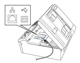
Carefully guide the USB cable into the trench as shown below, following the trench around and toward the back of the machine. Then, connect the cable to your Macintosh®.
