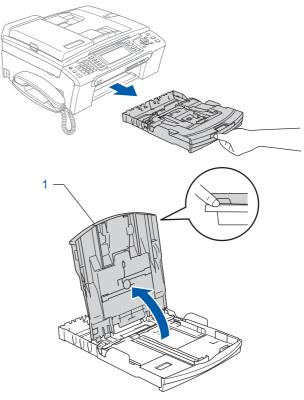
Press and slide the paper side guides (1) and paper length guide (2) to fit the paper size.
