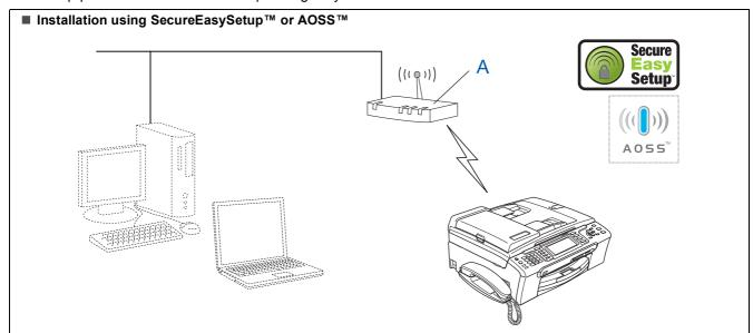
If your wireless access point (A) supports SecureEasySetup™ or AOSS™, you do not need to use a computer to configure the machine. The access point (router) and your machine can automatically negotiate using the SecureEasySetup™ or AOSS™ procedure.
