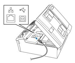
Carefully guide the network cable into the trench as shown below, following the trench around and toward the back of the machine. Then, connect the cable to your network.
