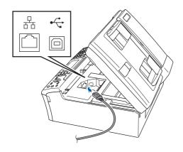
Carefully guide the network cable to the trench as shown below, following the trench around and toward the back of the machine.
