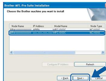
If your machine shows **APIPA** in the **IP Address** field, click **Configure IP Address** and enter an IP address for your machine that is suitable for your network.
