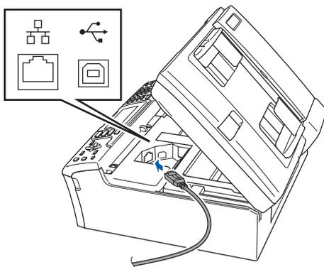
**4** Carefully route the network cable through the trench and out the back of the machine. Then, connect the cable to your network.
