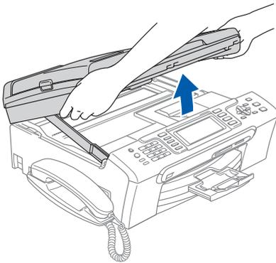
**3** Insert the network cable into the LAN socket marked with a
